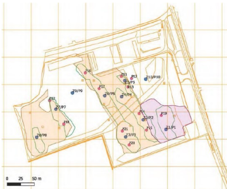
Figure 3-2: Mapped voids, 2019 geotechnical investigation © Terramech
