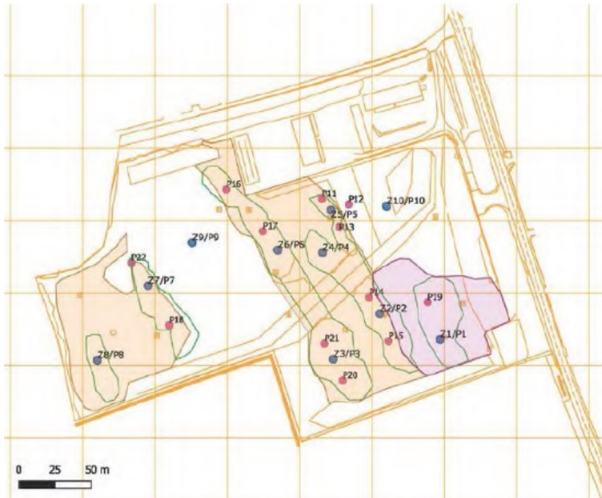
Figure 4-1: Deep voided ground in the chalk and shallow relaxed ground, 2019 geotechnical investigation © Zetica
